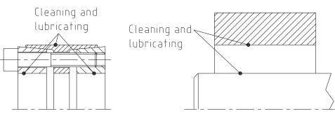
Illustration 5: Cleaning and lubricating the surfaces
