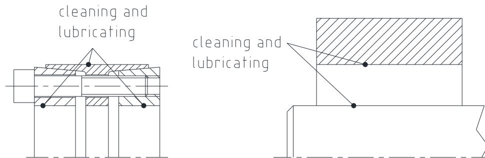
Illustration 5: Cleaning and lubricating the surfaces
