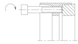
Illustration 9: Unscrewing the rear pressure ring
