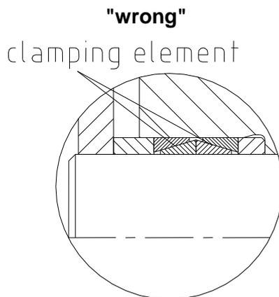
Illustration 6: Wrong installation of several clamping elements
