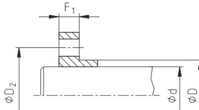
Illustration 2: Dimensions for calculation of pressure flange
