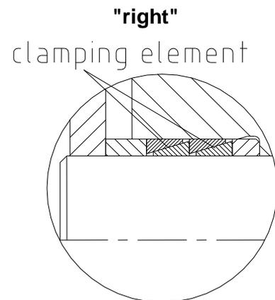
Illustration 7: Installation of several clamping elements
