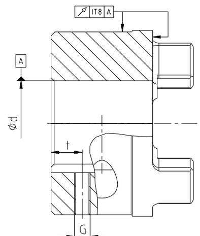
Illustration 9: Concentricity and axial runout
