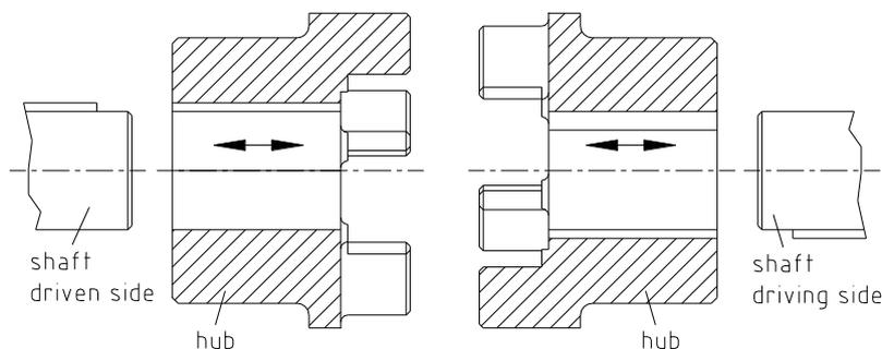
Illustration 5: Assembly of the hubs
