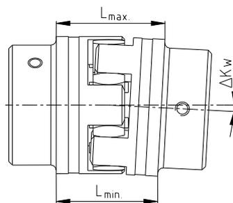
$$\Delta K_w = L_{1max.} - L_{1min.} \text{ [mm]}$$
