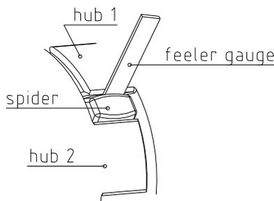
Illustration 14: Inspection of the limit of wear
