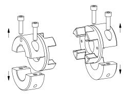
Illustration 22: Disassembly of half shells
