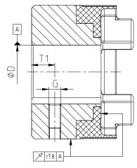
Illustration 14: Concentricity and axial runout (example: hub type 1c)
