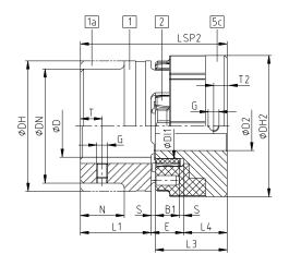
Illustration 4: Type EN (No. 081) - component 1, 1a, 1b: steel (St)
