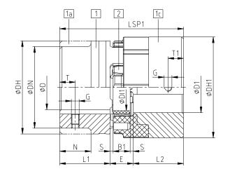
Illustration 1: Type GN (No. 080) - component 1, 1a, 1b: steel (St)
