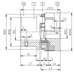
Illustration 5: Type EN (No. 081) - component 1, 1a, 1b: cast iron (GJL)
