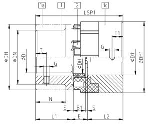
Illustration 2: Type GN (No. 080) - component 1, 1a, 1b: cast iron (GJL)
