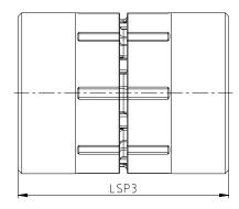
Illustration 17: Assembly of coupling (example: type GND)
