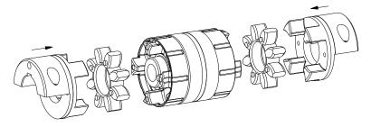
Illustration 23: Assembly of hub bodies, spiders and DKM spacer SP
