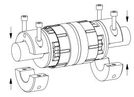
Illustration 24: Assembly of component assembly on the shafts
