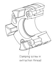
Illustration 22: Disassembly of clamping ring hub with clamping ring
