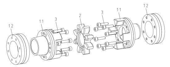
Illustration 17: ROTEX® GS clamping ring hub
