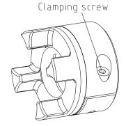
Illustration 20: Assembly of clamping hub
