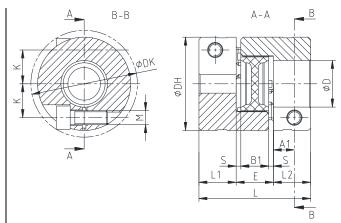
Illustration 7: ROTEX® GS 7, 9, 12, 14 and 19 Compact single slot (hub type 2.8/2.9)
