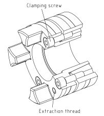
Illustration 21: Assembly of clamping ring hub with clamping ring
