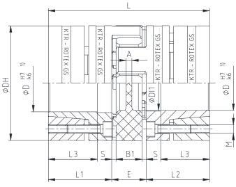
Illustration 9: ROTEX® GS, clamping ring hubs
