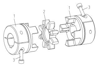
Illustration 14: ROTEX® GS clamping hub
