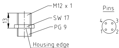
Illustration 10: Circular plug connection M12
